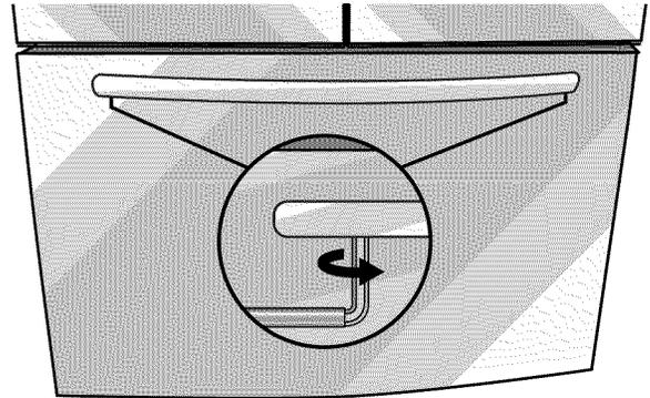
4. Using a left-to-right motion tighten the setscrew a quarter-turn at a time. Repeat until the screw feels tight.
