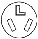
3-wire receptacle (10-30R)
