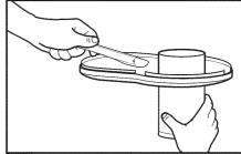
There may be pulp stuck to the underside of the lid. Use the flat side of the cleaning brush to carefully scrape the stuck pulp into the pulp container.
