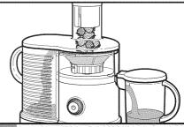
With motor running, place food into feed chute using the food pusher. As food is processed, the extracted juice will flow into the juice pitcher, and the separated pulp will flow into the pulp basket.
