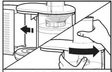
Remove pulp container. Grasp the feed chute on the Juicer lid and turn it counter-clockwise to remove it from the Juicer.
