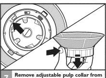
Remove adjustable pulp collar from the juice screen for cleaning:
