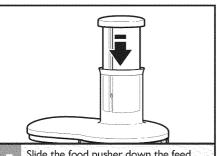
Slide the food pusher down the feed chute, aligning the groove in the food pusher with the protruding rib on the inside of the feed chute.
