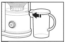
Place juice pitcher under the juice spout. Make sure juice spout is in the down position. **NOTE:** The lid of the juice pitcher comes equipped with a foam guard. To include the foam with your juice, simply remove the lid before pouring juice into your glass.
