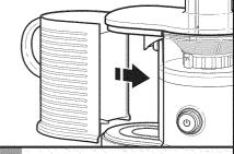
Slide the pulp basket into position under the long lid section until it rests against the motor body.
