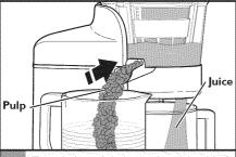
To make juice, the pulp chute should always be pushed in; this is the open positon. When the pulp chute is open, pulp created while juicing will flow through the pulp chute, separating it from the juice.
