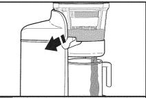
To make sauces, make sure the rubber gasket is in place, and sauce screen is installed. Pull the pulp chute out; this is the closed position. When the pulp chute is closed, the juice and fiber exit through the juice chute as a sauce.
