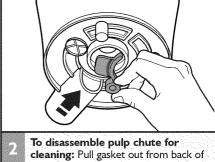
To disassemble pulp chute for cleaning: Pull gasket out from back of chute. Slightly pinch gasket hinge while sliding chute in towards the center of the juicing bowl.
