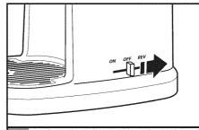
Pulp may build up on the screen and auger assembly and cause a jam. Clear the buildup by moving the power lever to OFF and then REV.
