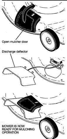
ACAUTION: Do not run your lawn mower without rear mulcher plate or plug in place or approved grass catcher in place. Never attempt to operate the lawn mower with the rear door removed or propped open.
