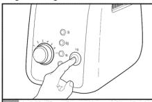
Press the TOAST/CANCEL (口会) button to begin toasting. The centering racks will adjust automatically to hold food upright. When toasting is complete, the End-of-Cycle signal will beep, the Toaster will shut off and raise the toast.
