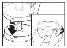
Fit the blade over the shaft in the center of the work bowl, rotate, and press down until it locks into operating position.
