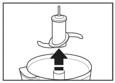
4. Holding the bowl as shown, twist bowl clockwise to unlock, and lift off the base.
