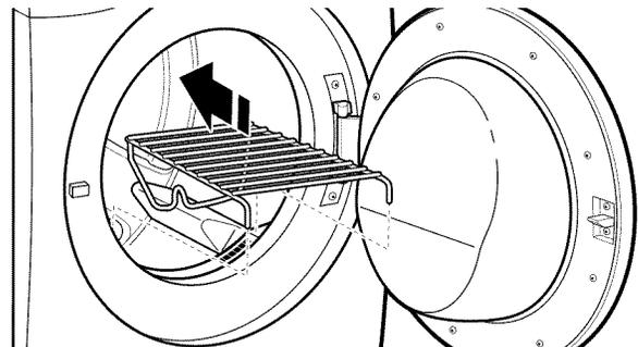
2. Align the two hooks on the front of the drying rack with the holes in the dryer door opening and press down fully into holes. Rest the rear support on the dryer back ledge.
