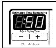
The temperature may be changed by pressing Temp until the desired dry temperature is lit. Once a cycle has started, the temperature can be changed after first pausing the cycle. Cycle time is estimated and may change throughout the cycle. Cycle time can not be changed on Steam Cycles.
