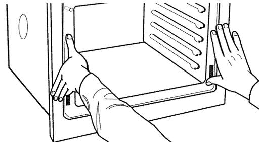
3. Push oven completely into the cabinet, and center the oven into the cabinet cutout.
