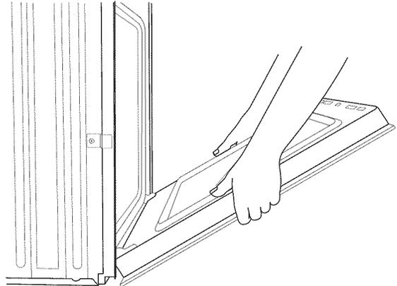
5. Using two hands, grasp the edges of the oven door. Lift and pull the oven door toward you and remove. You may need to gently shift door from side to side as you pull.
