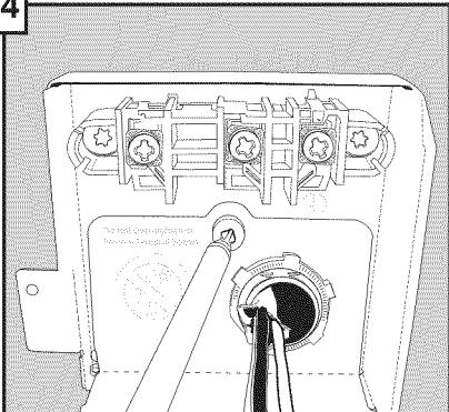
Place the assembled strain relief plate back into the junction box and re-attach the screw. Make sure the tab on the right side of the strain relief plate is outside the junction box as you slide it into place.
