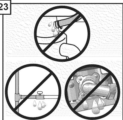
Attach water line to incoming hot water shut off valve. Turn on water and check for leaks. Turn power back on at fuse box. Start dishwasher and listen for water and pump for water distribution. Press Cancel/Reset to drain and check for leaks.
