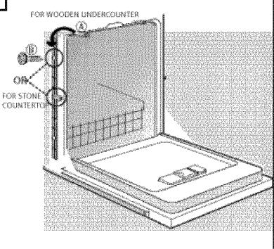
If your countertop is stone, detach mounting brackets (A) from the top and position them at either points on the side. Insert screw (B) through pre-positioned brackets on each side of the unit and attach the brackets.
