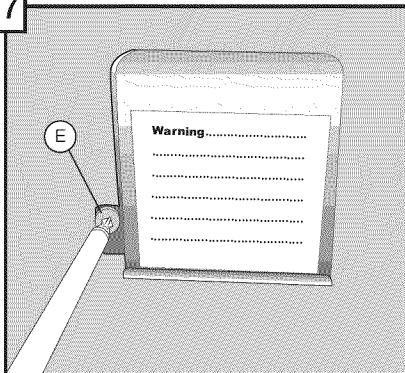
Replace junction box cover. Make sure the cover is seated behind the front lip of the strain relief plate. Attach the cover with the screw (Part E) from the installation kit.
