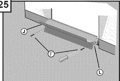
Slide screw (Part F), on the right side first, through the upper hole on the plastic toe panel (Part J), place washer (Part L) on the end of the screw, and attach the toe panel to the dishwasher by tightening the screw. Repeat for the left side.
