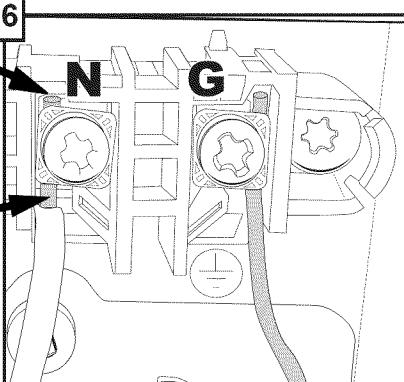
Make sure that the exposed (non-insulated) portion of each stripped wire shows above and below the terminal screw. Securely tighten the terminal screws, but do not over-tighten or damage may occur.
