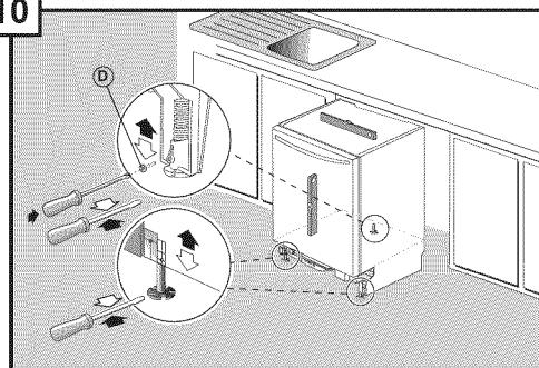
Pre-level unit before positioning under counter by turning feet clockwise to raise or counter-clockwise to lower. Maximum height the unit can be raised with feet fully extended is 34.5" (876.3 mm). Position unit under counter to verify that it is level. If adjustment is needed, remove unit from under counter and adjust as necessary. Once the unit is at a satisfactory height, insert leg leveler locking screw (Part D) in back foot. Step 18 will complete the leveling process.
