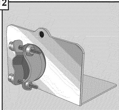
Attach the strain relief (not included) to the strain relief plate. The two screws on the back of the strain relief should be positioned as shown to prevent interferences during assembly. Tighten the strain relief lock nut to prevent the strain relief from turning.
