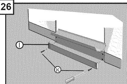
Attach screws (Part K) through the metal toe panel (Part I) to the lower holes of the plastic toe panel so it is flush with the floor.
