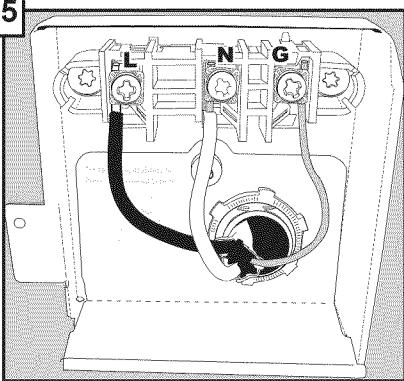
**Note:** Do not loosen or remove terminal screws! Damage may occur. Bend the wires so the exposed leads can reach the appropriate contacts. Insert the black (hot) wire into the left opening on the terminal strip marked "L", the white (neutral) wire in the middle opening of the terminal strip marked "N", and the bare copper or green (ground) wire into the right opening of the terminal strip marked "G". Hand tighten only. Do not use power tools.
