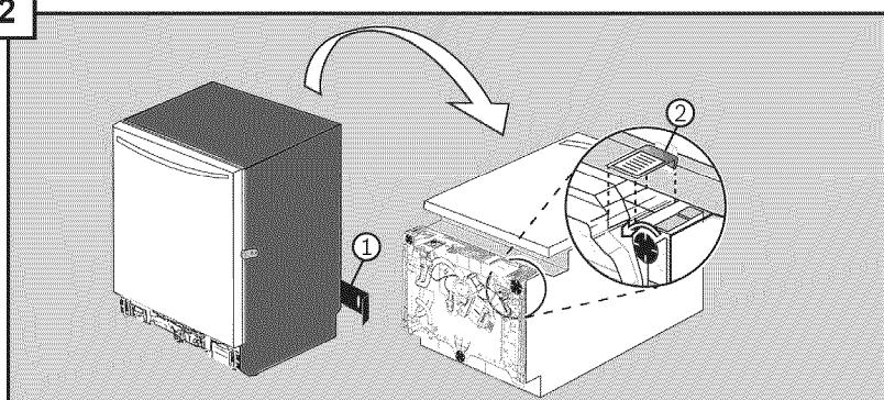
Remove the toe panel(s) (Part H or Parts I and J depending on model) (1) from the unit and retain for attachment to the front at a later time. Loosen the leg levelers slightly. Remove junction box cover and retain for later use (2). Discard the small piece of protective styrofoam.
