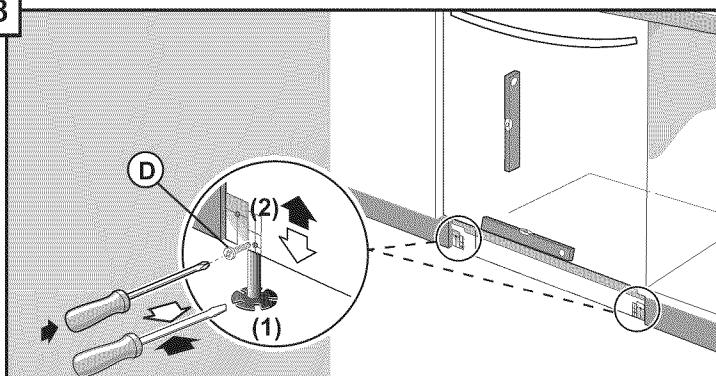
Level the dishwasher horizontally by turning feet (1) clockwise to raise or counter-clockwise to lower front of unit. Once level, (2) insert leg leveler locking screws (Part D) and tighten.
