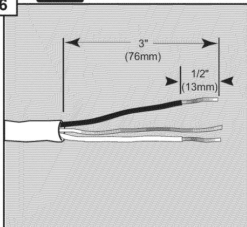
Strip outer casing of electrical wire to expose 3" (76.2 mm) of the inner wires. Then strip 1/2" (12.7 mm) casing from each individual wire.\*
