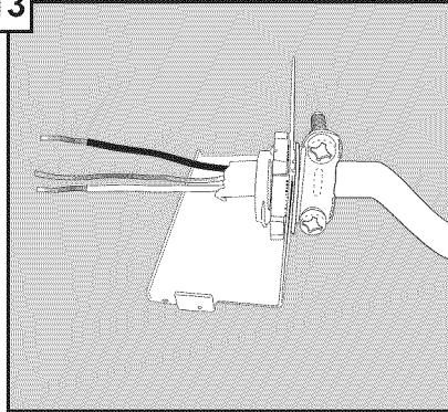
Pass wires through strain relief and plate. Tighten clamp around wires, oriented as shown. Bending the electrical cable as shown will ease installation of the strain relief plate.
