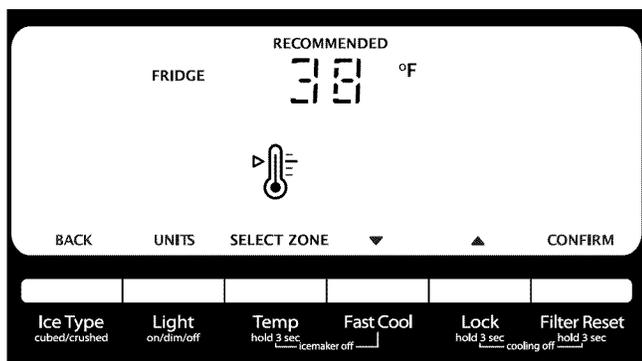
**NOTE:** To view Celsius temperatures, press the LIGHT button when adjust mode is activated. To return the display setting to Fahrenheit, press LIGHT again.
