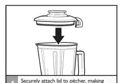
sure the handle on the lid aligns with the handle on the pitcher, as shown.
