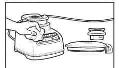
To clean the Blender base, control band, cord, lid, and ingredient cup: Unplug the Blender before cleaning. Wipe with a warm, damp cloth; wipe clean with a damp cloth, and dry with a soft cloth.
