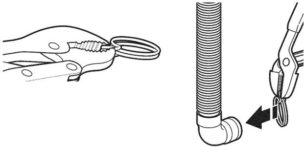
3. Squeeze clamp with pliers and slide elbow end of drain hose onto washer drain port and secure with clamp.
