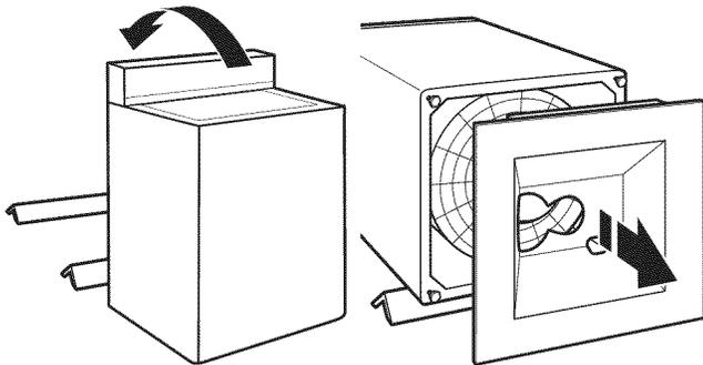
3. Remove tape from washer lid, open lid, and remove cardboard packing tray from tub. Be sure to remove all parts from tray.
