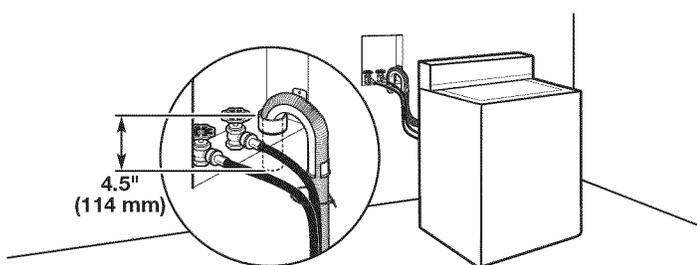
See requirements for floor standpipe drain system.
