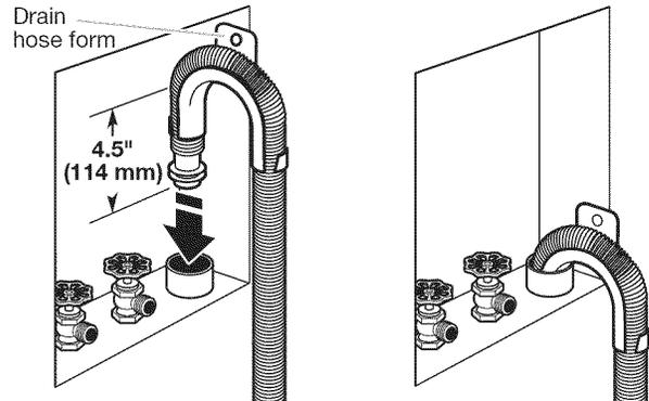
6. For floor drain installations, you will need to remove the drain hose form from the end of the drain hose. You may need additional parts with separate directions. See "Tools and Parts."
