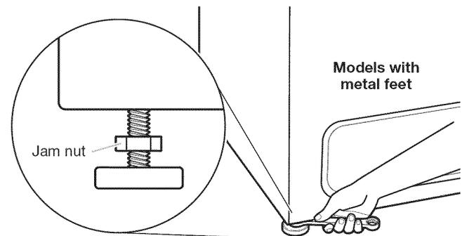
3. On models with metal feet, when washer is level, use a  $9/16"$  or 14 mm open-end or adjustable wrench to turn jam nuts counterclockwise on leveling feet tightly against washer cabinet.
