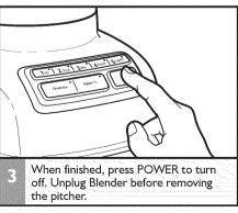
**NOTE:** The Blender will operate only when pressing the POWER button (Power LED will flash) before selecting the desired speed.
