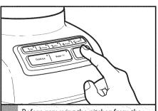
Before removing the pitcher from the base, always press POWER to stop the flashing lights and unplug the power
