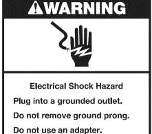
Do not use an extension cord. Failure to follow these instructions can result in death, fire, or electrical shock,
