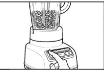
To clean the pitcher while attached to the base: Keep the pitcher on the Blender base, fill half full with warm (not hot) water, and add I or 2 drops of dishwashing liquid. Put the lid on the pitcher, press the STIR speed setting, and run the Blender for 5 to I0 seconds. Remove the pitcher and rinse with warm water.
