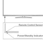
$\begin{tabular}{ll} \textbf{Power/Standby Indicator:} Light up in red when the TV is in standby mode. Light out when the TV is on. \end{tabular}$
