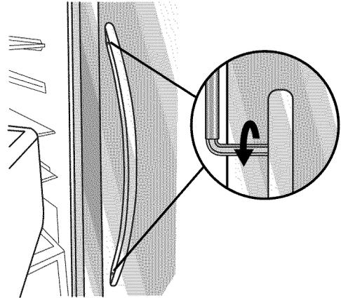
5. Using a clockwise motion, tighten the setscrew until it begins to contact the shoulder screw.
