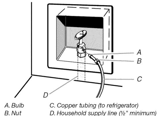
4. Now you are ready to connect the copper tubing to the shutoff valve. Use 1/4" (6.35 mm) OD soft copper tubing to connect the shutoff valve and the refrigerator.
