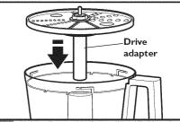
With the work bowl installed, slide the drive adapter onto the power shaft. Then install the work bowl cover, being sure it locks into place. You may need to turn the disc/adapter until it drops into place.
