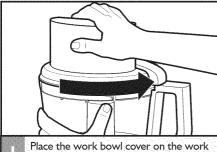
Place the work bowl cover on the work bowl with the feed tube just to the left of the work bowl handle. Grasp the feed tube and turn the cover to the right until it locks into place.
