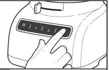
The pulse control allows precise control of the duration and frequency of processing. It's great for jobs which require a light touch. Just press and hold the PULSE Button to start processing at high speed, and release it to stop.
