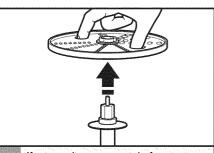
If using a disc, remove it before removing the bowl. Holding the disc by the 2 finger grips, lift it straight up, then remove the adapter.
