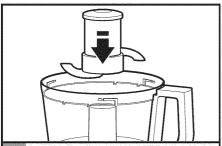
Place the blade on the power shaft. Rotate the blade so it falls into place on the power shaft.
