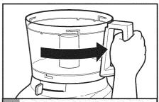
Grasp the work bowl handle and turn the bowl counterclockwise to lock it on the base.
