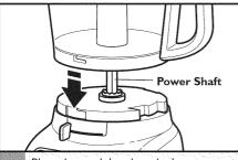
Place the work bowl on the base, aligning the raised portion with the indentation on the base. The center hole should fit over the power shaft.
