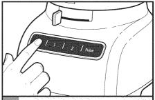
When finished, press the "O" (Off) button. The indicator light will go out and the blade or disc will slow to a stop.
