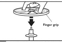
Hold the reversible shredding disc by the 2 finger grips with the desired shredding side facing UP. Insert the disc adapter into the hole in the bottom of the disc.
