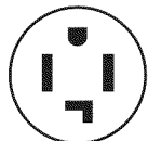
4-wire receptacle (14-30R)
