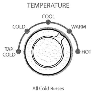
Once you select a cycle, select the desired wash temperature by turning the Temperature knob to the appropriate setting based on your load. All rinses are cold.
