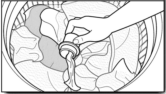
During the final rinse, wait until the washer has completed filling, press the START/Pause button to pause the washer. Lift the lid and add the measured, recommended amount of liquid fabric softener. Do not use more than the recommended amount. Close the lid and press the START/Pause button again to restart the washer.
