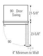
**NOTE:** Right-hand models illustrated. Allow the same clearances on the opposite side for left-hand fresh food models ZIF1240 and ZIFS240 only. Models ZIB1240 and ZIBS240 are not available with left-hand door swing.
