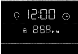
Figure 29: Clean cycle in progress
