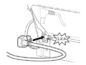
An optional power cord is available, which plugs into the power module and replaces the junction box with cord provided with the dishwasher (SMZPC002UC – service # 00747210). To install it, feed it through the adjacent cabinet hole, plug it into the rear of the power module until it "clicks" and plug it into the customer receptacle (outlet).
