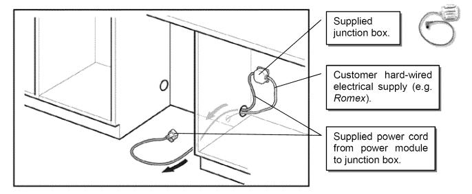
**NOTE**: Screws are not provided to mount the junction box inside the adjacent cabinet.
