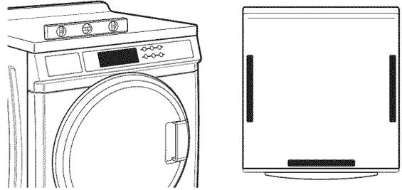
If the washer is against a wall, move the washer out slightly before tipping back. If the washer is not level, first prop the front with a wood block and adjust the feet as necessary; then prop the back and adjust feet as necessary. Repeat this step until washer is level.
