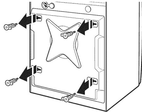
4. Once all 4 bolts are removed, discard the bolts and spacers. Then push the plug back into the back of the washer and pull the power cord through the left opening of the rear panel and close the hole with the attached cap.
