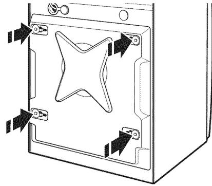
3. Once the bolt is loose, move it to the center of the hole and completely pull out the bolt, including the plastic spacer covering the bolt.
