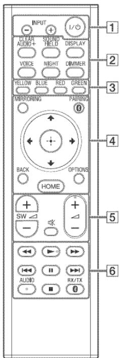
AUDIO, ▶, and ▲ + buttons have a tactile dot. Use the tactile dot as a reference when operating the remote control.
