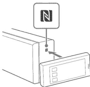
Follow the on-screen instructions displayed on the remote device, and complete the procedure for BLUETOOTH connection. When the BLUETOOTH connection is established, the blue LED indicator on the front panel lights up.
