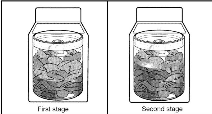
Your new washer saves energy by using lower water levels and reduced wash temperatures, as compared to traditional top-load washers. During the first stage of the wash cycle, it is normal for some of the load to be above the water line. The second stage adds the correct amount of water based on the load size. This washer automatically adjusts the water level to the load size. No water level selector is needed.
