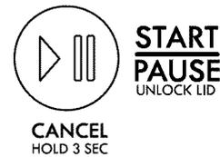
Press the START/PAUSE/Unlock Lid button to start the wash cycle. When the cycle has finished, the Cycle Complete status light will light. Promptly remove garments after cycle has completed to avoid odor, reduce wrinkling, and rusting of metal hooks, zippers, and snaps.
