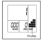
When you select a preset workout, the duration of the workout will appear in the upper display and a profile of the resistance levels of the workout will scroll across the center display.
