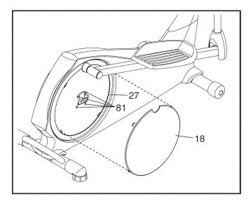
Then, remove the M8 x 12mm Screws (81) from the Right Pedal Disc (27), and gently rotate the Right Pedal Disc out of the way.
