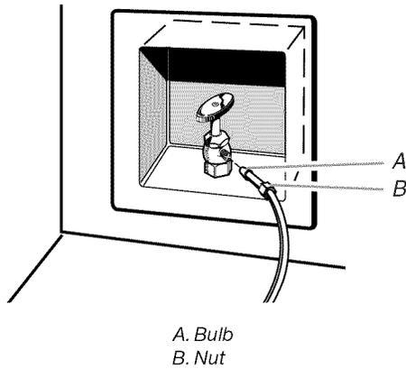
3. Now you are ready to connect the copper tubing. Use 1/4" (6.35 mm) O.D. soft copper tubing for the cold water supply.
