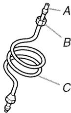
4. Place the free end of the tubing into a container or sink, and turn on main water supply and flush out tubing until water is clear. Turn off shutoff valve on the water pipe.
