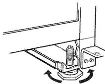
5. Push up on the top rear of the ice maker and locate the leveling legs that are on the bottom rear of the ice maker.
