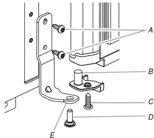
A. Hex-head hinge screw    D. Hinge pin
