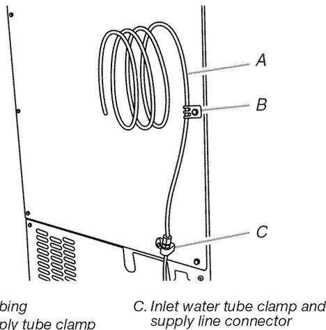
6. Remove and discard the short, black plastic tube from the end of the water line inlet.
