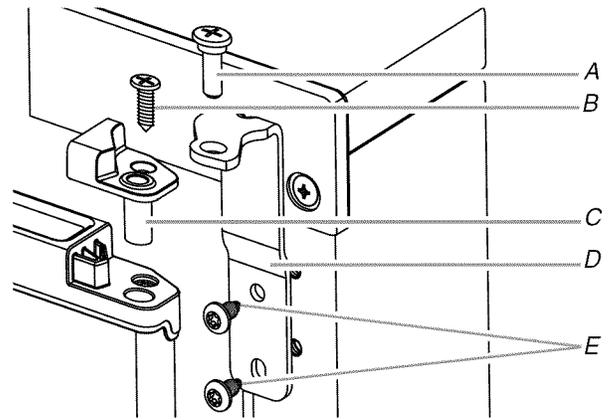
A. Hinge pin    D. Hinge
