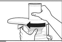
Place the juicer lid over the bowl housing so that the long lid section is slightly to the right of the pulp exit chute. Grip the feed chute, turning the lid clockwise until it locks into place.
