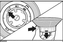
Remove adjustable pulp collar from the juice screen for cleaning: Turn collar to "unlock." Press spring button and pull collar down, removing it from the screen.
