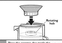
Place the ceramic disc inside the juicing bowl on top of the rotating hub. Rotate the disc until the tabs on the inside of the collar match up with the notches on the hub and the disc settles easily into place.
