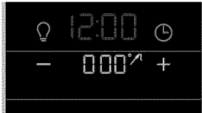
Figure 24: Probe inserted and ready to set temperature
