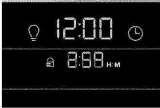
Figure 35: Clean cycle in progress
