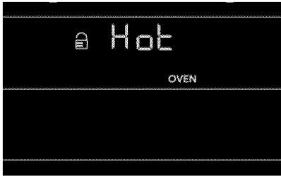
Figure 36: Hot oven after clean with door still locked
