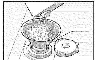
**Warning:** Never fill the salt dispenser with detergent. It will destroy the water softening system. To prevent corrosion, refill with salt and immediately begin any cycle.
