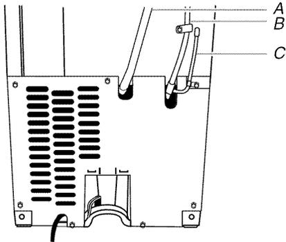
A. Drain hose (drain pump models only)
