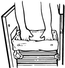
**NOTE:** The ram can and will tear improperly installed bags.
