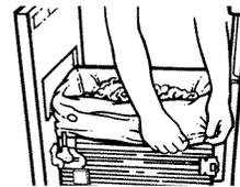
3. Release drawer side latch. Tilt drawer to the right. This releases pressure on the bag making it easier to remove the bag.
