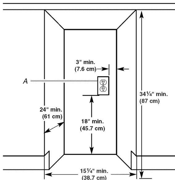
A. Grounded electrical outlet must be a minimum of 3" (7.6 cm) away from surrounding cabinets or nearby walls as shown. It can be placed either to the left or the right side of the product.
