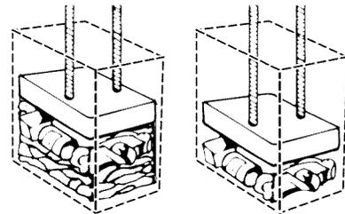
Load bulky trash, bottles, and cans in the center of the drawer. Bottles or cans not placed in the center may become caught between the ram and the drawer. The Drawer Monitor Switch will sense a "misload" and causes the ram to return to the "up" position without compacting.
