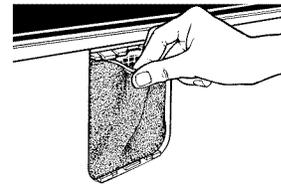
4. To replace air filter, push the replacement filter into place.
