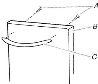
A. 2 screws inserted into holes from inside of drawer
