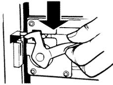
4. Hold the drawer latch open and tilt the side of the drawer out until the lock clears the drawer front. Remove the drawer side by lifting it out of the drawer.
