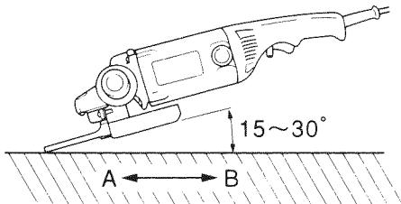
**NOTE:** The wheel provided (resinoid wheel) is rated as Class A grain and #36 grain size. It is most suitable for heavy grinding of steel and other types of materials.
