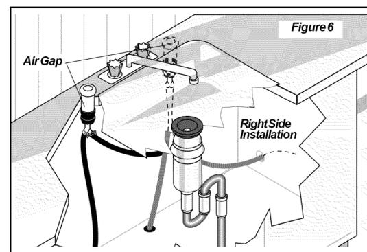
3. If you connect to a sink trap, local codes may require you to install an air gap kit, (not included). The drain hose will be routed from dishwasher to air gap inlet as shown in Figure 6. An air gap kit is available from a plumbing supply store. NOTE: If the drain hose is installed through the floor, an air gap is necessary.
