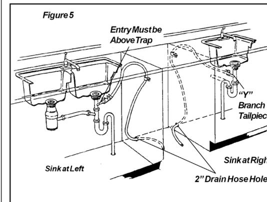
2. If you connect to a sink drain, entry will need to be above trap. A "Y" branch tailpiece and connector kit, not included, will make this method easier and includes all needed fittings and instructions. See Figure 5.
