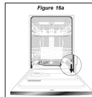
2. Close and latch door while holding both sides.
