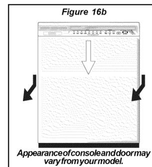
4. Place door where it will not get scratched or damaged while completing installation.
