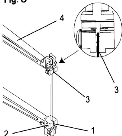
4. Insert the other end of the blade into the upper blade holder slot (3-Fig. O) and then tighten the tension knob (5-Fig. P).
