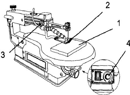
1. Lay out or secure design to workpiece (1).
