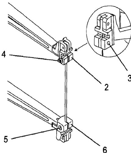
3. Tilt the table to 0° and tighten the table lock knob (7-Fig. N). Loosen the lower blade holder lock screw (5-Fig. M) under the table on the left side of the lower blade holder (6-Fig. M) with the supplied T-wrench by turning counterclockwise.
