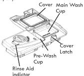
If the cover is closed on the Main Wash Cup open by pressing the Cover Latch.
