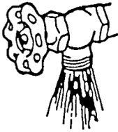
Put a flat washer from the parts bag into each end of the four inlet hose couplings. Be sure flat washers are *firmly* seated.
