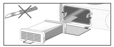
Rinse the heat exchanger and the cap on all sides with a jet of water to completely remove all of the lint and fluff.
