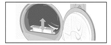
The filter should be cleaned after or before every drying process. Cleaning the filter reduces the drying time and saves energy.
