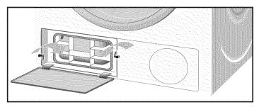
5. Pull out the heat exchanger cap.
