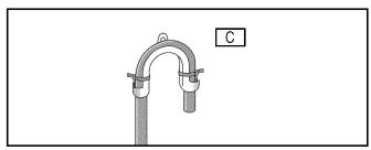
Secure hose and/or elbow as shown below. Sink "D" or floor "E".
