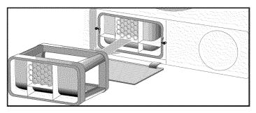
6. Remove the heat exchanger.
