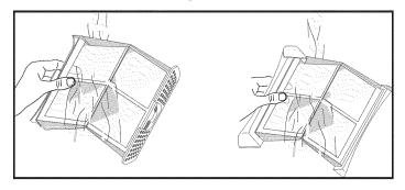
The filter must be dried thoroughly before being placed back into dryer.
