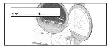
The **E-Nr.** (model number) and the **FD** (serial) number are found on the rating plate label.
