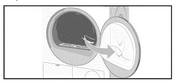
2. The deposit on the sensors can easily be removed by wiping the sensors (the two bars next to the lint filter) with a cloth and a little white vinegar.
