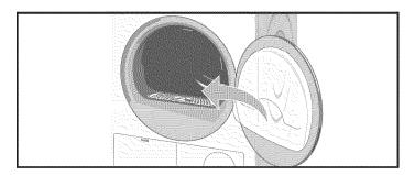
**NOTICE:** Severely dirty or clogged lint filter should be rinsed under warm running water.
