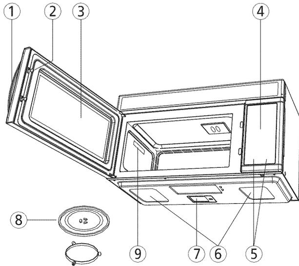
**1. DOOR HANDLE** - Pull to open door. Door must be securely latched for oven to operate.
