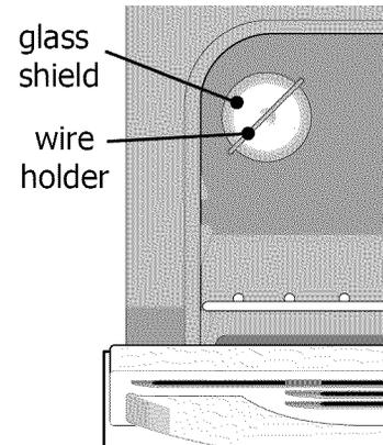
The glass shield should always be in place to protect and shield the oven interior light whenever using the oven.
