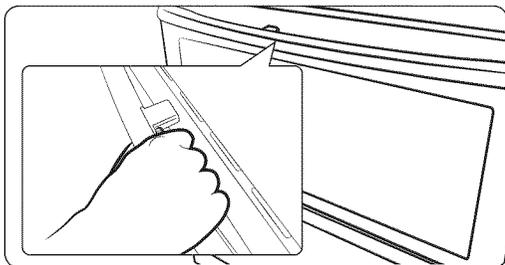
1. Hold the handle and the lever, press the lever to release the door latch, and then pull the handle.
