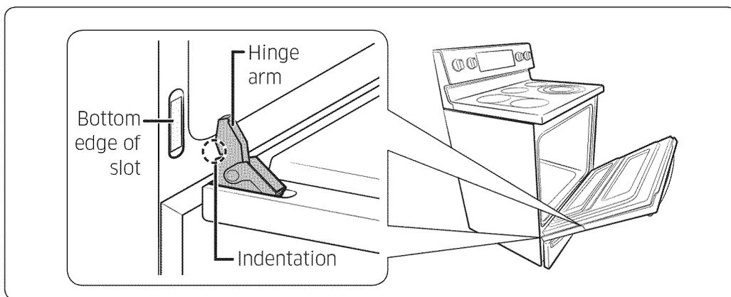
3. Open the door fully. If the door will not open fully, the indentation is not inserted correctly in the bottom edge of the slot.
