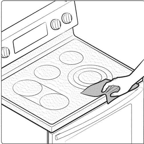
To clean the seal around the edges of the glass, lay a wet cloth on it for a few minutes, then wipe clean with a nonabrasive cleaner.
