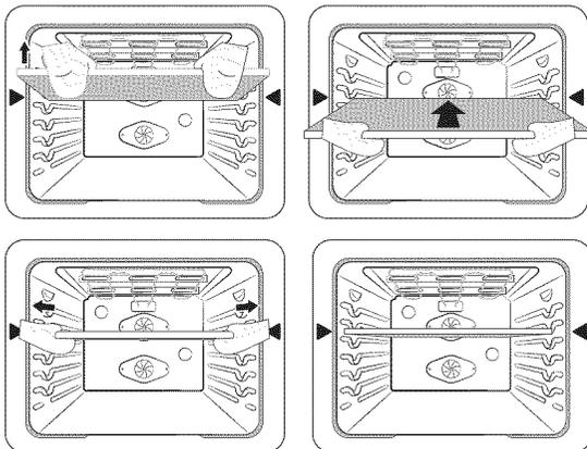
1. Insert the partition into the 5th rack position of the cavity.
