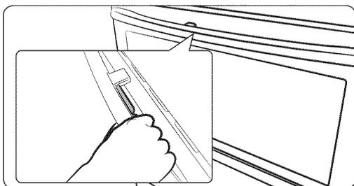
1. Hold the lever-less area of the handle, and then pull.
