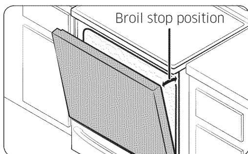
Leave the door open at the broil stop position. The door will stay open by itself, yet the proper temperature is maintained in the oven.
