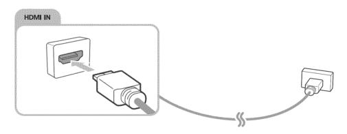
Set Edit Device Type to DVI PC for a computer connected with a HDMI-to-DVI cable, and PC for a computer connected with HDMI cable. Also, set Edit Device Type to DVI Devices for an A/V device with a HDMI-to-DVI cable.
