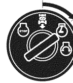
Engine "On" Position (Normal Operating)
