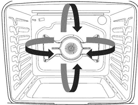
True convection adds an electric element around the convection fan to enhance the cooking performance. This feature enables three-rack baking in your range. Use the following Convection Options chart as a guide.
