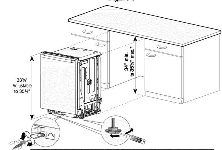
1. Measure height of cabinet opening from underside of countertop to floor.
