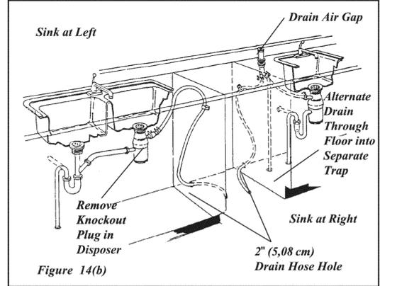
The drain hose loop must be at least 32" (80 cm) high from the floor to insure proper drainage.
