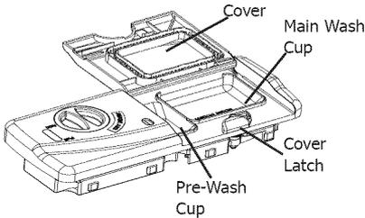
If the cover is closed on the Main Wash Cup open by pressing the Cover Latch.
