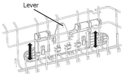
To lower the upper rack, press the lever and push down on the rack.
