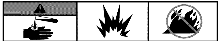
Battery acid is corrosive, explosive and flammable
