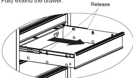
**Lever Style** - Lift or lower (depending on the slide) the release lever on both sides, (this allows the slides to ride over the stops). Pull out to remove.
