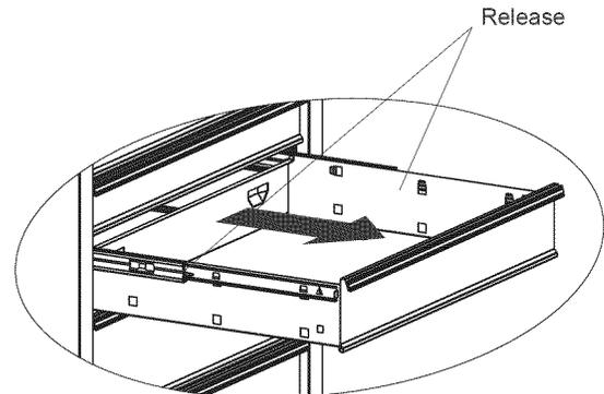
**Lever Style** - Lift or lower (depending on the slide) the release lever on both sides, (this allows the slides to ride over the stops.) Pull out to remove.
